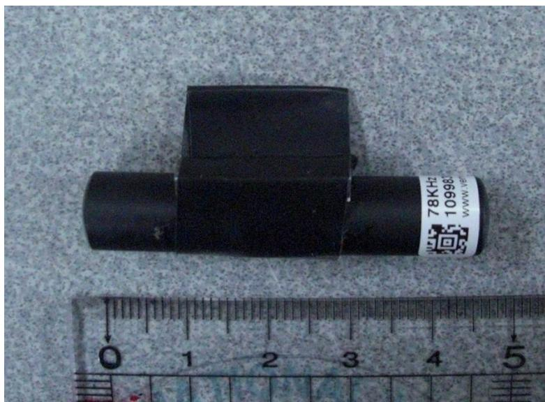
Fig. 3. Acoustic tag to measure the behaviour of mackerel (*Scomber japonicus*) in the cage net.
