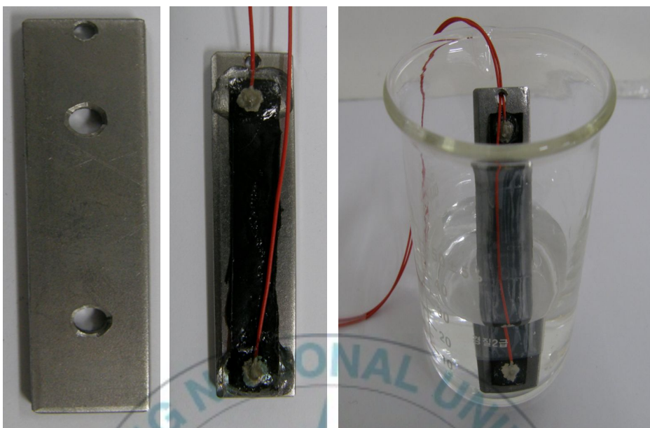
Fig.VI-2 A sample of CNT / Nafion composite (5wt%) sensor electrode (20x50x0.02mm) on metal specimen.
