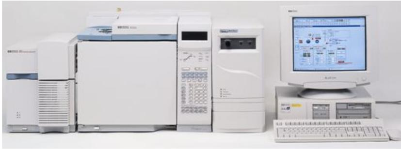
Fig. 3.8. Pre-concentrator and GC/MS analysis apparatus.
