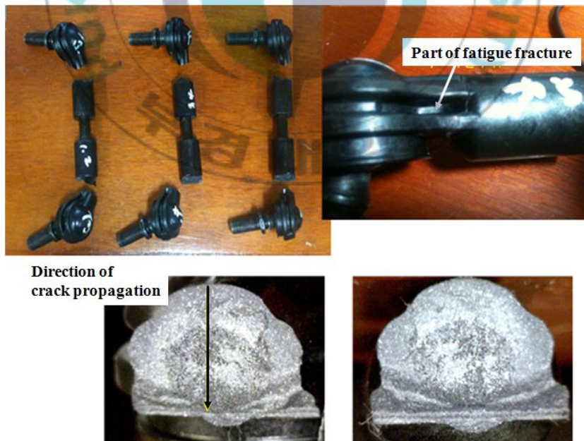
Fig. 2.28 Appearance of fatigue fractured surface
