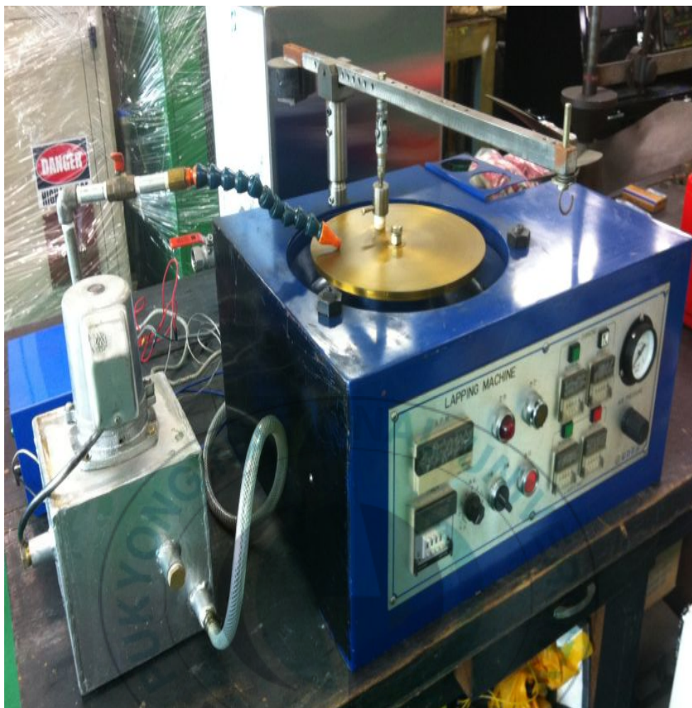
Fig. 9 Pin on disk system of friction coefficient and wear test apparatus
