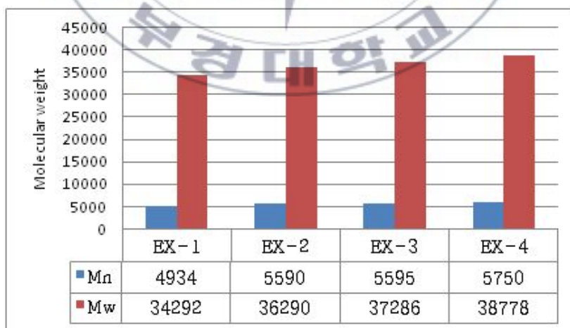
Fig 9. Molecular weights of copolymer synthesized with various composition.
