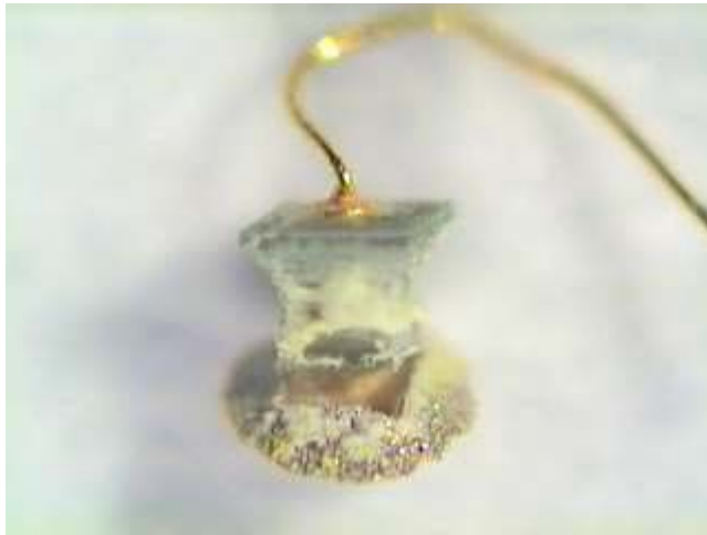
Fig. 3 Lived chip caused by reflow of thermal paste chip attach
