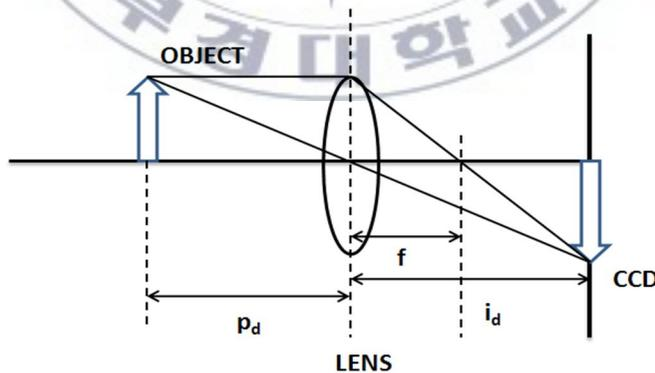
Figure 1-1 Geometry of a Stereoscopic Camera Lens System.
