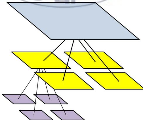
Figure 4-5 Quadtree Segmentation of an Image.
