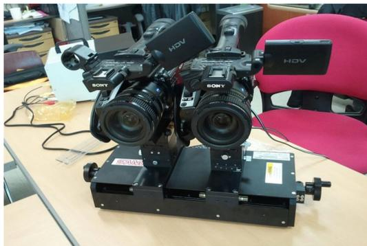
Figure 3-4 Stereoscopic (3D) Camera Rig.
