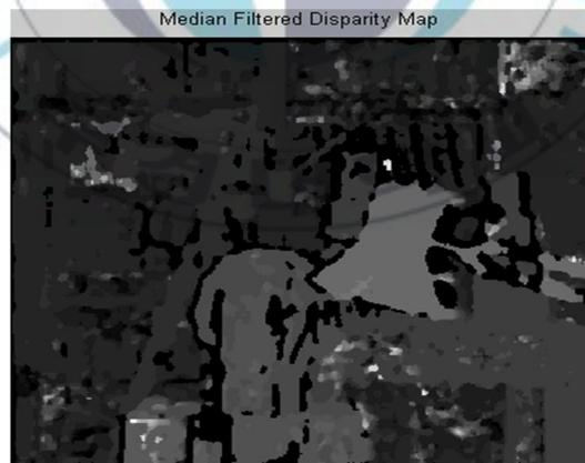
Figure 3-12 Median Filtered Disparity Map.
