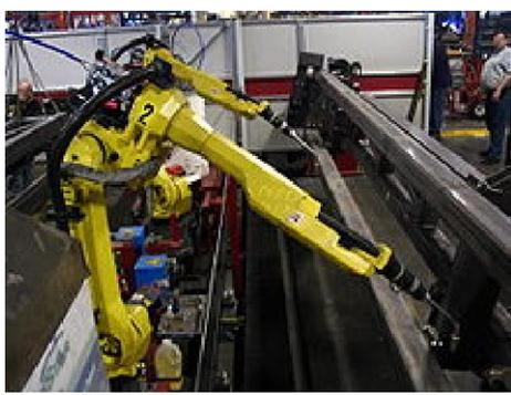
Fig. 1.2 Set of six-axis robots used for welding
