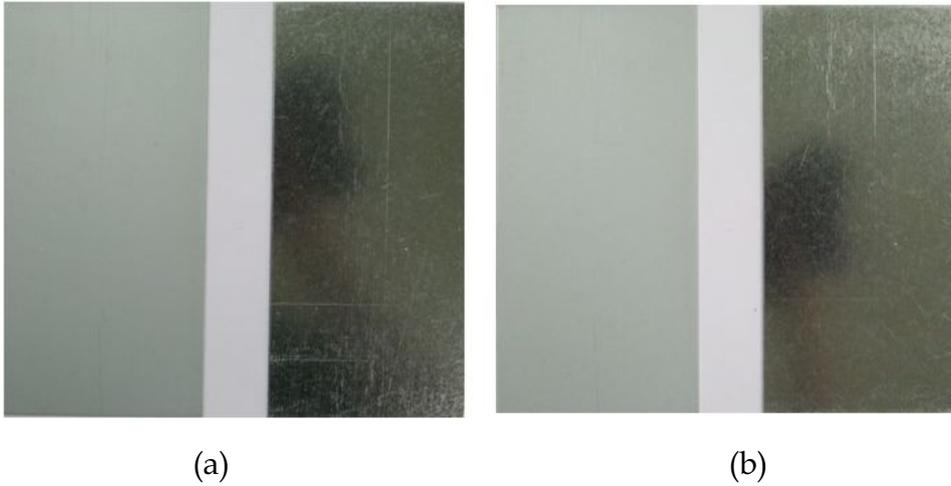
**Fig. 3.9 Stability test of LRO-317 coating specimens**
