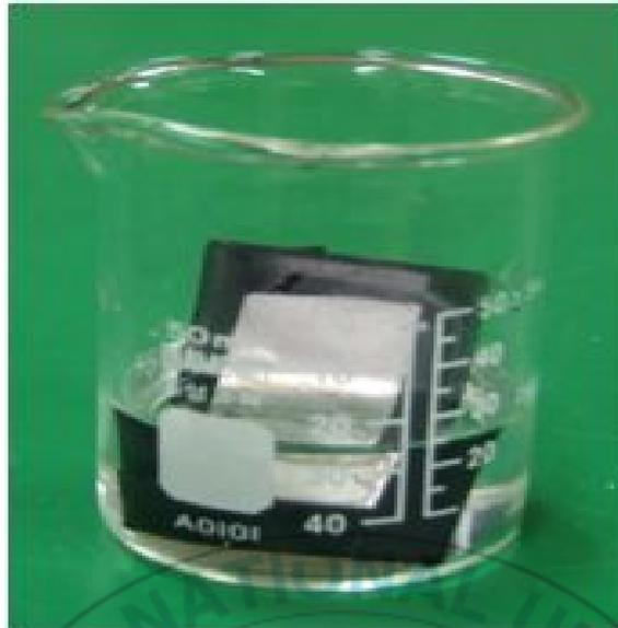
**Fig. 4.3 Immersion test of the coating specimen**
