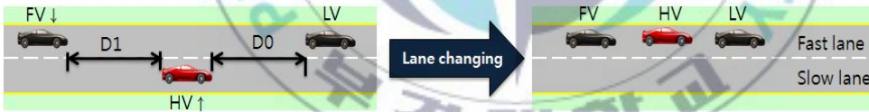
Figure 4.6. ASV of lane changing from the slow lane to the fast lane.
