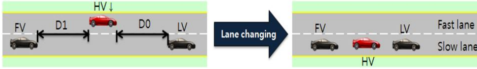
Figure 4.2. Manual vehicle of lane changing from the fast lane to the slow lane.
