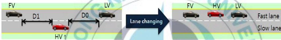
Figure 4.3. Manual vehicle of lane changing from the slow lane to the fast lane.
