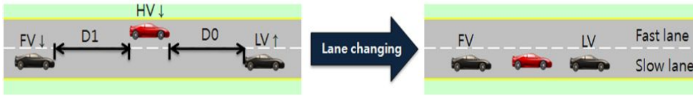
Figure 4.5. ASV of lane changing from the fast lane to the slow lane.
