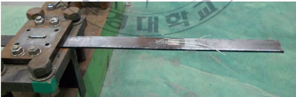
Figure 3.5 Experimental setup of cantilever beam
