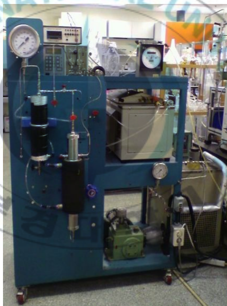
Fig. 2.1. Photograph and schematic diagram of SC-CO 2 extraction process.
