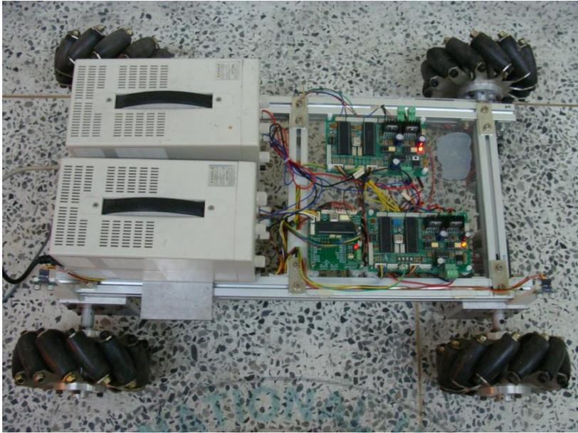
Fig. 2.2 Omni-directional Mobile Robot
