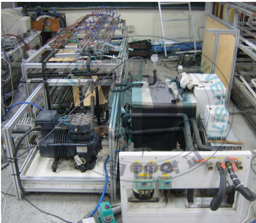
Photo. 2.1 Experimental apparatus for CO 2 system.
