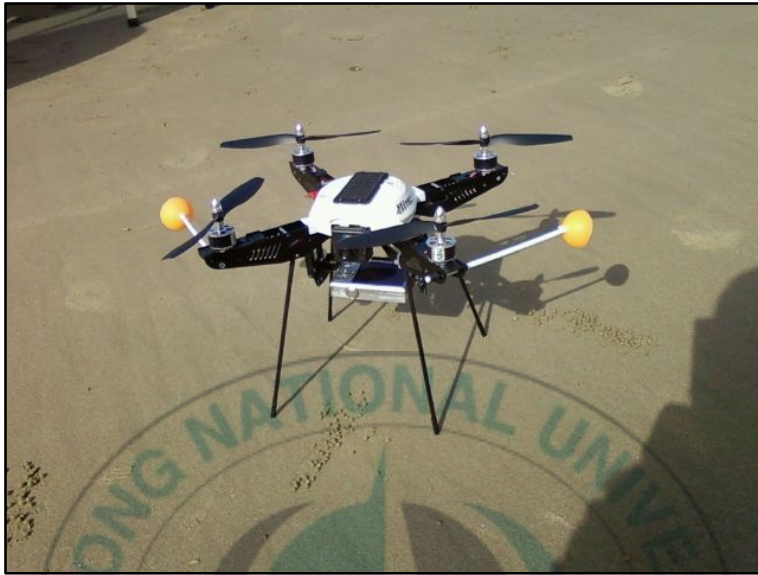
Fig. 3.1.1 The pilotless aircraft for image acquisition
