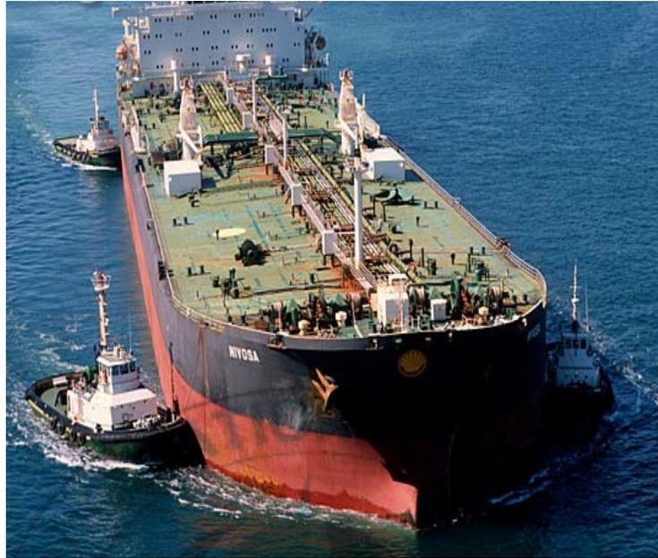
Fig.1.3. Ship maneuvering for berthing with assistance of tugboats.
